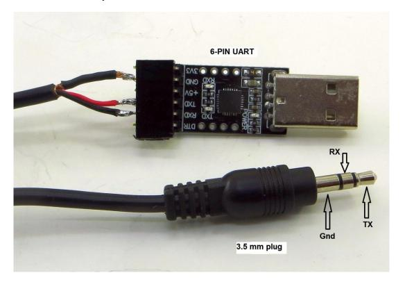
I used a 6-pin in-line header as a socket for the UART module. A piece of clear heat-shrink tubing helps protect the assembly as shown below:
